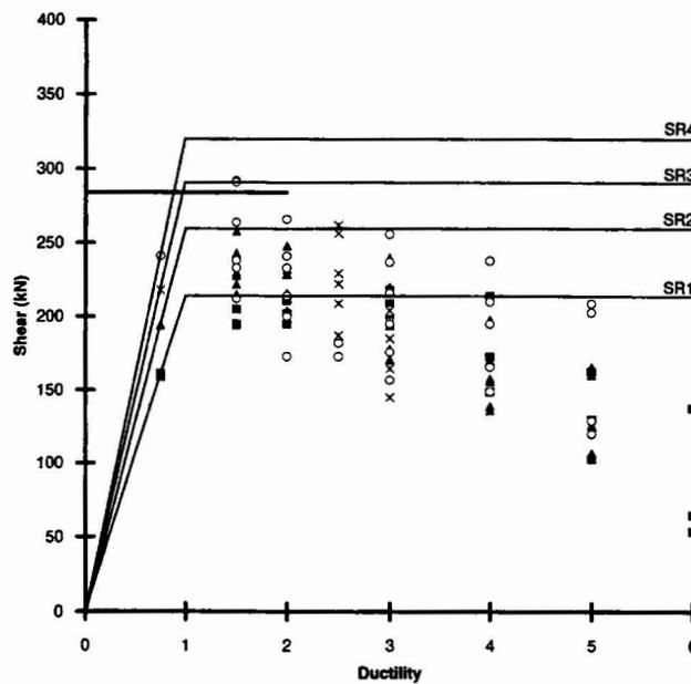
Fig. 5 — Peak shear force values at each load cycle.
