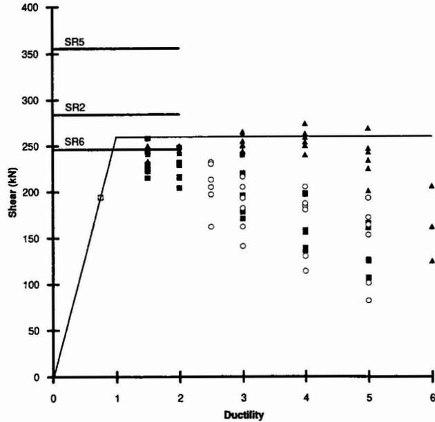
Fig. 6 — Peak shear force values at each load cycle.
