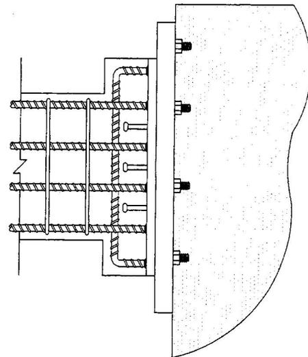
Fig. 2 — Specimen boundary conditions.
