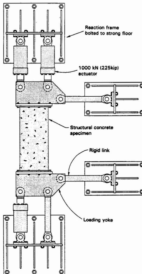
Fig. 1 — Plan view of element tester.
