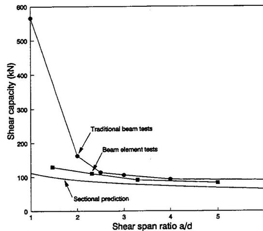
Fig. 3 — Influence of shear span on beam tests.
